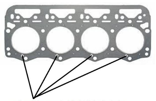
Install water jacket support tubes in heads & block at these locations
